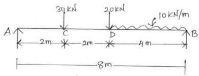
b) Draw bending moment and shear force diagram for the overhanging beam shown in the figure. Clearly indicate point of contraflexure.8 M
