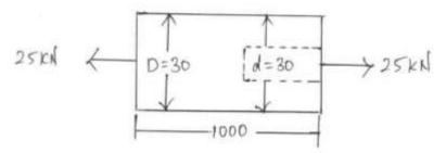
b) The steel bar of uniformly varying diameter shown in the figure is held between two Unyielding supports at room temperature. What is the maximum stress induced in the bar, if temperature rises by 30°C? Take  $Es=2\times10^5 N/mm^2$  and  $\alpha s=12\times10^{-6}/°C$ . 6 M
